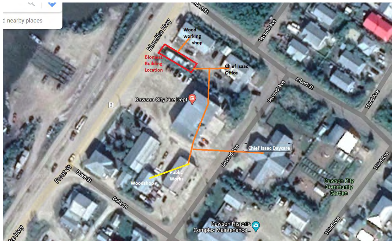
Figure : A google map of the City Fire Hall/Admin Building, City Public Works Building, City Woodshop, Chief Isaac Office, Tr'ondëk Hwëch'in Daycare and Chief Isaac wood working shop. The most likely location for a biomass facility is highlighted in red. The buildings that have potential for biomass heating have orange and yellow lines running to them. A detailed design would be required to accomplish this work. An energy assessment of other buildings to be connected to the biomass must be conducted prior to detailed design to ensure that they are using energy efficiently and to prevent oversizing the biomass system.
