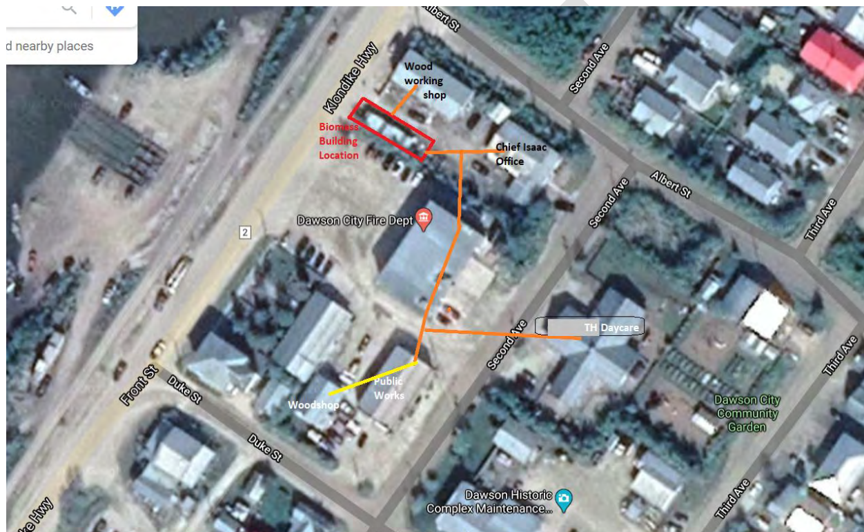
Figure 4: A google map of the City Fire Hall/Admin Building, City Public Works Building, City Woodshop, Chief Isaac Office, Tr'ondëk Hwëch'in Daycare and Chief Isaac wood working shop. The most likely location for a biomass facility is highlighted in red. The buildings that have potential for biomass heating have orange and yellow lines running to them. A detailed design would be required to accomplish this work. An engineering/energy assessment and optimally recommissioning of other buildings to be connected to the biomass must be conducted prior to detailed design to ensure that they are using energy efficiently and to prevent oversizing the biomass system.
