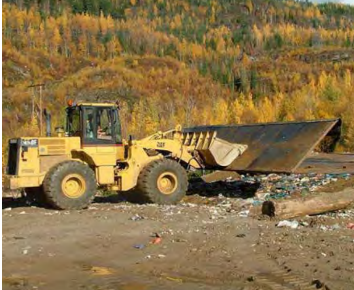
Figure 5-2: Rigid Steel Plate Alternate Cover System
