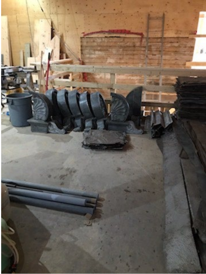
Figure 16: Restored exterior cladding material
