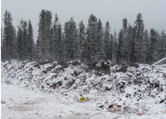
Figure 6-5: Windrow Composting in the Sub-Arctic (note steam coming from top of pile)
