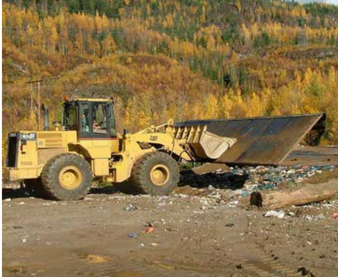
Figure 5-2: Rigid Steel Plate Alternate Cover System
